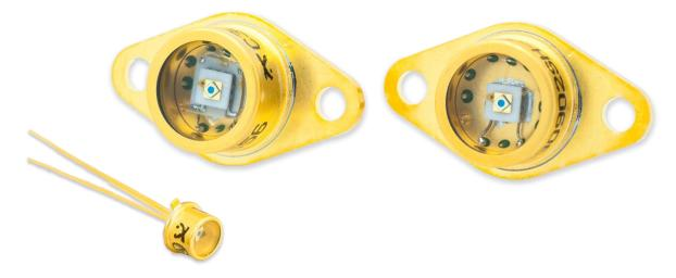
Excelitas' C30902SH Avalanche Photodiodes are high speed, large area Silicon APDs that provide high responsivity at low noise. They are specially selected to be used either in Geiger Mode ( $V_{op} > V_{BD}$ ) for detection of single photons or Linear Mode ( $V_{op} < V_{BD}$ ) with Gains up to 250.
